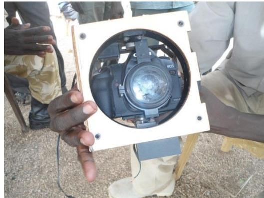
**The pictures show a Sudanese UAV which crash-landed in Delami County in April 2014. The picture on the right shows the camera mounting used on the UAV.**
